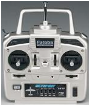
A typical hobby transmitter. This one has four channels(can control four functions).
