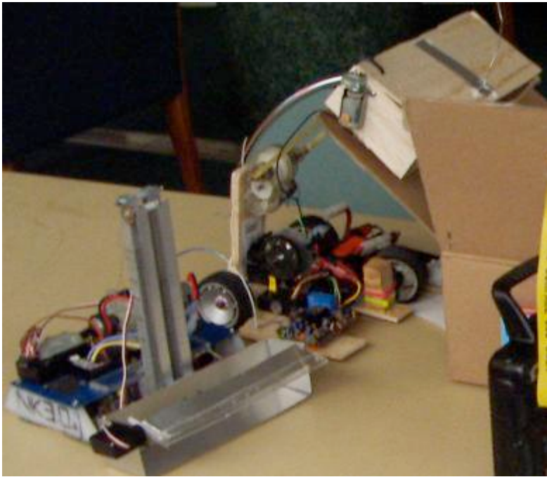
North Gwinnett's other 2005 entry is in the background, a hypotenuse design with a large flap door and utterly overpowered arm motor.
